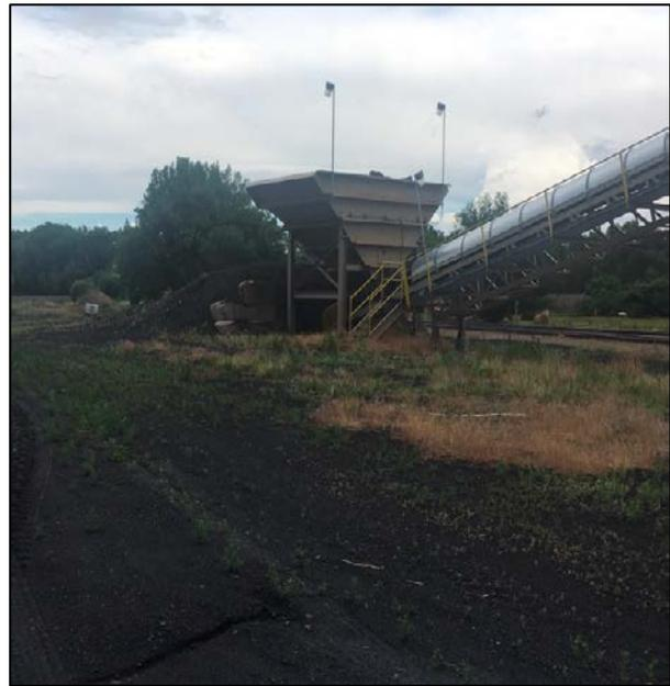
Image: Feeding system into the rail loadout.
